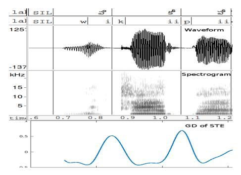
Figure 4.9: An example of a Telugu utterance that shows syllable boundary detection with GD of STE. The first and second panels show the syllable and phone transcriptions respectively. The boundary of the syllables *wi*, and *kii* corresponds to a peak in the GD of STE.
