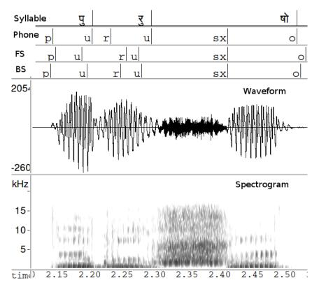
Figure 4.2: Bootstrap segmentation. The first panel shows the syllable transcription (in UTF-8 encoding), the second panel shows the actual phone boundaries, the third panel shows the phone boundaries obtained with flat start segmentation (5 hours of data) and the fourth panel shows the phone boundaries obtained with bootstrap segmentation (5 hours of data, out of which 10 minutes was manually labelled).
