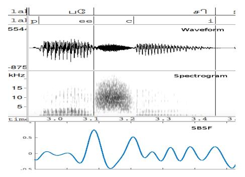
Figure 4.14: An example of a Tamil utterance that shows syllable boundary detection with SBSF. The first and second panels show the syllable and phone transcriptions respectively. SBSF gives a peak near the boundary of the syllables *pee*, and *ci* (first phone of the syllable *ci* is an affricate *c*).
