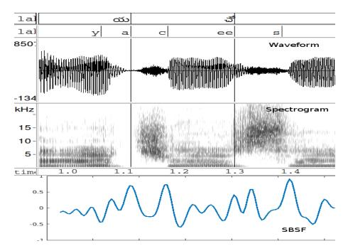
Figure 4.13: An example of a Telugu utterance that shows syllable boundary detection with SBSF. The first and second panels show the syllable and phone transcriptions respectively. SBSF gives a peak near the boundary of the syllables ya, and cee (first phone of the syllable *cee* is an affricate c).
