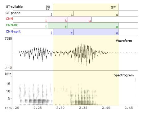
Figure 5.13: An example from part of a Tamil utterance, where syllable  $\mathfrak{F}_{J}$  (tu) is highlighted, with phone boundaries obtained using CNN-HMM and CNN-HMM with boundary correction.
