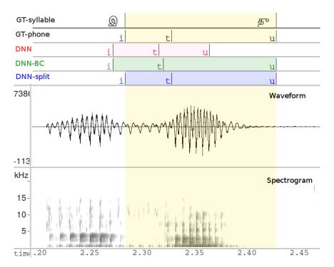
Figure 5.12: An example from part of a Tamil utterance, where syllable  $\mathfrak{F}$  (tu) is highlighted, with phone boundaries obtained using DNN-HMM and DNN-HMM with boundary correction.
