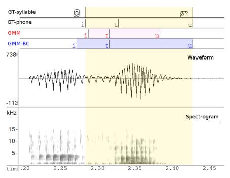
Figure 5.11: An example from part of a Tamil utterance, where syllable  $\mathfrak{g}_{J}$  (tu) is high-lighted, with phone boundaries obtained using GMM-HMM and GMM-HMM with boundary correction.
