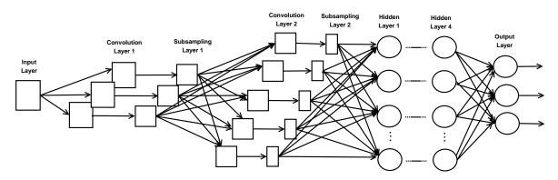
Figure 5.3: Schematic diagram of CNN
