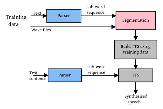
Figure 2.1: Block diagram of text-to-speech synthesis system
