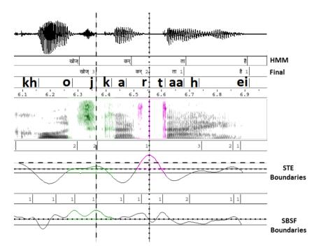
Figure 4.17: An example of a Hindi utterance that shows boundary correction using STE and SBSF.
