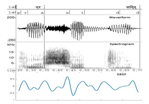
Figure 4.11: An example of a Hindi utterance that shows syllable boundary detection with SBSF. The first and second panels show the syllable and phone transcriptions respectively. SBSF gives a peak near the boundary of the syllables *pra*, and *sid* (first phone of the syllable *sid* is a fricative *s*).
