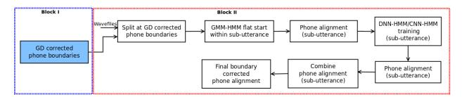
**Figure 5.7:** Block diagram of DNN-HMM/CNN-HMM segmentation with boundary correction: Non-iterative approach. The *GD corrected phone boundaries* are obtained using the procedure shown in Block I of Figure 5.6.
