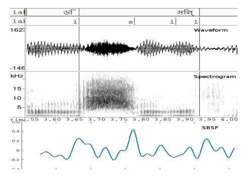
Figure 4.12: An example of a Bengali utterance that shows syllable boundary detection with SBSF. The first and second panels show the syllable and phone transcriptions respectively. SBSF gives a peak near the boundary of the syllables dxi, and sil (first phone of the syllable sil is a fricative s).
