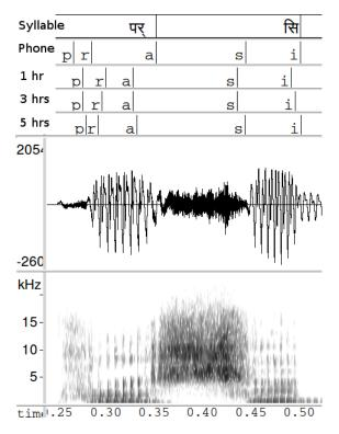
Figure 5.5: HMM flat start segmentation with different hours of training data. The first panel shows the syllable transcription (in UTF-8 encoding), the second panel shows the actual phone boundaries, the third, fourth, and fifth panels show the phone boundaries obtained with 1 hour, 3 hours, and 5 hours of data respectively.
