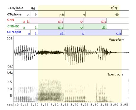
Figure 5.10: An example from part of a Hindi utterance, where syllable शोध् (shodh) is highlighted, with phone boundaries obtained using CNN-HMM and CNN-HMM with boundary correction.
