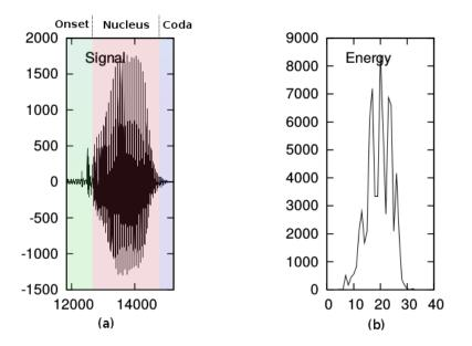
Figure 4.4: Waveform and energy plots of a syllable. X-axis correspond to time in samples at a sampling rate of 16 kHz (fig a). The energy plot shows the corresponding number of frames in a syllable (fig b).
