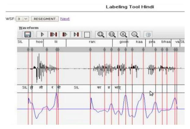
Figure 4.3: Semi-automatic labeling tool for manual correction of syllable boundaries obtained with GD segmentation. The tool has an option to play the waveform fully or as segments, and to insert, delete, or move the syllable boundaries. It also provides the facility to play with a tuning parameter called window scale factor (WSF) (discussed in Section 4.4) to control the number of syllable boundaries given by GD.
