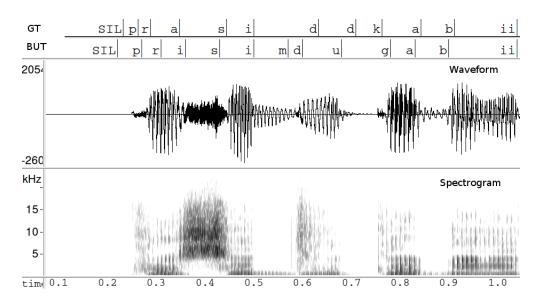
Figure 5.1: Phone boundaries obtained for a Hindi speech utterance using BUT phone recognizer. The first panel shows the actual phone boundaries (denoted as ground truth (GT), the second panel shows the phone boundaries obtained with BUT recognizer. Comparison between first and second panels shows the presence of insertion and substitution errors.
